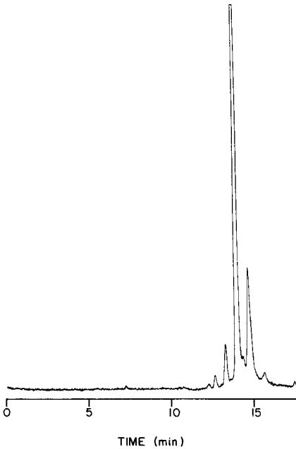
Fig. 4. Zone electrophoretic separation of bovine pancreatic trypsinogen on surface-modified 50\text{ cm} \times 75\text{ }\mu\text{m} I.D. fused silica. The sample concentration was 0.2\% (w/v) in 0.05\text{ M} phosphate buffer. Injection time, 5\text{ s} at 10\text{ kV} ; electrophoresis at 10\text{ kV} .
